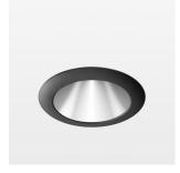
Recessed downlight with LED, rated life of the LED L80/B10 > 500000 h, colour rendering index CRI > 90, chromaticity tolerance 2 SDCM (initial), reflector with homogeneous light distribution pattern, diffuser lens, translucent, darklight reflector, aluminium, metallised, highgloss, luminaire head die-cast aluminium, powder-coated, mounting ring die-cast aluminum, front ring and coverblind plastic, black, separate driver unit
