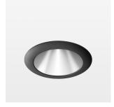
Recessed downlight with LED, rated life of the LED L80/B10 > 50000 h, chromaticity tolerance 2 SDCM (initial), reflector with homogeneous light distribution pattern, diffuser lens, translucent, darklight reflector, aluminium, metallised, highgloss, luminaire head die-cast aluminium, powder-coated, mounting ring die-cast aluminum, front ring and coverblind plastic, black, separate driver unit
