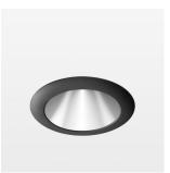
Recessed downlight with LED, rated life of the LED L80/B10 > 50000 h, chromaticity tolerance 3 SDCM (initial), reflector with homogeneous light distribution pattern, diffuser lens, translucent, darklight reflector, aluminium, metallised, highgloss, luminaire head die-cast aluminium, powder-coated, mounting ring die-cast aluminum, front ring and coverblind plastic, black, separate driver unit
