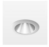
Recessed downlight with LED, rated life of the LED L80/B10 > 50000 h, colour rendering index CRI > 80, chromaticity tolerance 2 SDCM (initial), reflector with homogeneous light distribution pattern, diffuser lens, translucent, darklight reflector, aluminium, metallised, highgloss, luminaire head die-cast aluminium, powder-coated, mounting ring die-cast aluminum, front ring and coverblind plastic, white, separate driver unit
