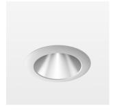
Recessed downlight with LED, rated life of the LED L80/B10 > 500000 h, colour rendering index CRI > 90, chromaticity tolerance 2 SDCM (initial), reflector with homogeneous light distribution pattern, diffuser lens, translucent, darklight reflector, aluminium, metallised, highgloss, luminaire head die-cast aluminium, powder-coated, mounting ring die-cast aluminum, front ring and coverblind plastic, white, separate driver unit
