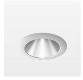
Recessed downlight with LED, rated life of the LED L80/B10 > 500000 h, colour rendering index CRI > 96, chromaticity tolerance 3 SDCM (initial), reflector with homogeneous light distribution pattern, diffuser lens, translucent, darklight reflector, aluminium, metallised, highgloss, luminaire head die-cast aluminium, powder-coated, mounting ring die-cast aluminum, front ring and coverblind plastic, white, separate driver unit
