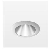
Recessed downlight with LED, rated life of the LED L80/B10 > 50000 h, chromaticity tolerance 2 SDCM (initial), reflector with homogeneous light distribution pattern, diffuser lens, translucent, darklight reflector, aluminium, metallised, highgloss, luminaire head die-cast aluminium, powder-coated, mounting ring die-cast aluminum, front ring and coverblind plastic, white, separate driver unit
