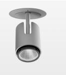
Semi-recessed luminaire with LED, rated life of the LED L80/B10 > 50000 h, chromaticity tolerance 2 SDCM (initial), , reflector with circular light distribution pattern, reflector pure aluminium 99,99% in MIRO-Silver®, segmented and faceted, exchangeable reflector unit in high-sheen black plastic, with glass cover, luminaire head die-cast aluminium, powder-coated, rotation angle 330°, swivel angle +90°/-90°, luminaire housing die-cast aluminium, powder-coated, stratosilver, separate driver unit
