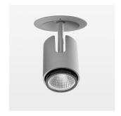
Semi-recessed luminaire with LED, rated life of the LED L80/B10 > 50000 h, chromaticity tolerance 3 SDCM (initial), , reflector with circular light distribution pattern, reflector pure aluminium 99,99% in MIRO-Silver®, segmented and faceted, exchangeable reflector unit in high-sheen black plastic, with glass cover, luminaire head die-cast aluminium, powder-coated, rotation angle 330°, swivel angle +90°/-90°, luminaire housing die-cast aluminium, powder-coated, stratosilver, separate driver unit
