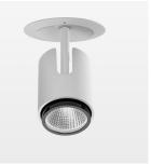
Semi-recessed luminaire with LED, rated life of the LED L80/B10 > 50000 h, chromaticity tolerance 3 SDCM (initial), , reflector with circular light distribution pattern, reflector pure aluminium 99,99% in MIRO-Silver®, segmented and faceted, exchangeable reflector unit in high-sheen black plastic, with glass cover, luminaire head die-cast aluminium, powder-coated, rotation angle 330°, swivel angle +90°/-90°, luminaire housing die-cast aluminium, powder-coated, stratowhite, separate driver unit
