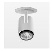
Semi-recessed luminaire with LED, rated life of the LED L80/B10 > 50000 h, chromaticity tolerance 3 SDCM (initial), , reflector with circular light distribution pattern, reflector pure aluminium 99,99% in MIRO-Silver®, segmented and faceted, exchangeable reflector unit in high-sheen black plastic, with glass cover, luminaire head die-cast aluminium, powder-coated, rotation angle 330°, swivel angle +90°/-90°, luminaire housing die-cast aluminium, powder-coated, stratowhite, separate driver unit
