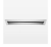
Recessed lumionaire for grid ceiling with LED, rated life of the LED L80/B10 > 50000 h, color rendering index CRI > 90, chromaticity point tolerance 3 SDCM (initial), Reflector with asymerical light distribution pattern, 99.99% pure aluminium reflector made of MIRO-SILVER®, aluminium luminaire housing and frame, anodized, separate driver unit.
