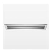
Recessed lumionaire for grid ceiling with LED, rated life of the LED L80/B10 > 50000 h, color rendering index CRI > 90, chromaticity point tolerance 3 SDCM (initial), Reflector with asymerical light distribution pattern, 99.99% pure aluminium reflector made of MIRO-SILVER®, aluminium luminaire housing and frame, anodized, separate driver unit.
