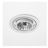
Recessed luminaire with LED, rated life of the LED L80/B10 > 50000h, colour rendering index CRI > 80, chromaticity tolerance 2 SDCM (initial), axially symmetrical reflector with circular light distribution pattern, 99,99% pure aluminium, segmented and faceted, cardanic, incl. glass cover, sheet metal powder coated, separate driver unit
