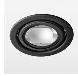
Recessed luminaire with LED, rated life of the LED L70/B10 > 50000 h, chromaticity tolerance 3 SDCM (initial), reflector with circular light distribution pattern, reflector pure aluminium 99,99% in MIRO-Silver®, swivel angle +25°/-25°, luminaire housing sheet steel, powder-coated, stratoblack, separate driver unit
