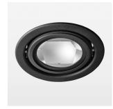
Recessed luminaire with LED, rated life of the LED L80/B10 > 50000 h, chromaticity tolerance 2 SDCM (initial), reflector with oval light distribution pattern, reflector pure aluminium 99,99% in MIRO-Silver®, luminaire head die-cast aluminium, powder-coated, swivel angle +25°/-25°, luminaire housing sheet steel, powder-coated, stratoblack, separate driver unit
