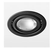
Recessed luminaire with LED, rated life of the LED L80/B10 > 50000 h, chromaticity tolerance 3 SDCM (initial), reflector with oval light distribution pattern, reflector pure aluminium 99,99% in MIRO-Silver®, luminaire head die-cast aluminium, powder-coated, swivel angle +25°/-25°, luminaire housing sheet steel, powder-coated, stratoblack, separate driver unit
