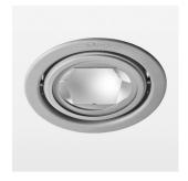
Recessed luminaire with LED, rated life of the LED L80/B10 > 50000 h, chromaticity tolerance 2 SDCM (initial), reflector with oval light distribution pattern, reflector pure aluminium 99,99% in MIRO-Silver®, luminaire head die-cast aluminium, powder-coated, swivel angle +25°/-25°, luminaire housing sheet steel, powder-coated, stratosilver, separate driver unit
