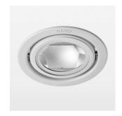
Recessed luminaire with LED, rated life of the LED L80/B10 > 50000 h, chromaticity tolerance 2 SDCM (initial), reflector with oval light distribution pattern, reflector pure aluminium 99,99% in MIRO-Silver®, luminaire head die-cast aluminium, powder-coated, swivel angle +25°/-25°, luminaire housing sheet steel, powder-coated, stratowhite, separate driver unit
