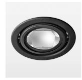
Recessed luminaire with LED, rated life of the LED L80/B10 > 50000 h, chromaticity tolerance 2 SDCM (initial), reflector with circular light distribution pattern, reflector pure aluminium 99,99% in MIRO-Silver®, luminaire head die-cast aluminium, powder-coated, swivel angle +25°/-25°, luminaire housing sheet steel, powder-coated, stratoblack, separate driver unit
