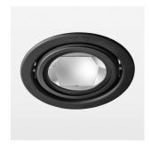
Recessed luminaire with LED, rated life of the LED L80/B10 > 50000 h, chromaticity tolerance 2 SDCM (initial), reflector with circular light distribution pattern, reflector pure aluminium 99,99% in MIRO-Silver®, luminaire head die-cast aluminium, powder-coated, swivel angle +25°/-25°, luminaire housing sheet steel, powder-coated, stratoblack, separate driver unit
