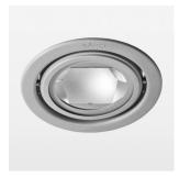
Recessed luminaire with LED, rated life of the LED L80/B10 > 50000 h, chromaticity tolerance 2 SDCM (initial), reflector with circular light distribution pattern, reflector pure aluminium 99,99% in MIRO-Silver®, luminaire head die-cast aluminium, powder-coated, swivel angle +25°/-25°, luminaire housing sheet steel, powder-coated, stratosilver, separate driver unit
