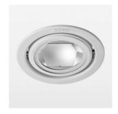
Recessed luminaire with LED, rated life of the LED L80/B10 > 50000 h, chromaticity tolerance 2 SDCM (initial), reflector with circular light distribution pattern, reflector pure aluminium 99,99% in MIRO-Silver®, luminaire head die-cast aluminium, powder-coated, swivel angle +25°/-25°, luminaire housing sheet steel, powder-coated, stratowhite, separate driver unit
