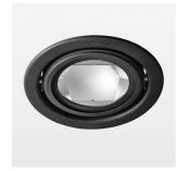
Recessed luminaire with LED, rated life of the LED L80/B10 > 50000 h, colour rendering index CRI > 80, chromaticity tolerance 3 SDCM (initial), reflector with circular light distribution pattern, reflector pure aluminium 99,99% in MIRO-Silver®, swivel angle +25°/-25°, luminaire housing sheet steel, powdercoated, stratoblack, separate driver unit
