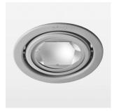
Recessed luminaire with LED, rated life of the LED L80/B10 > 50000 h, colour rendering index CRI > 80, chromaticity tolerance 3 SDCM (initial), reflector with circular light distribution pattern, reflector pure aluminium 99,99% in MIRO-Silver®, swivel angle +25°/-25°, luminaire housing sheet steel, powdercoated, stratosilver, separate driver unit
