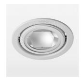
Recessed luminaire with LED, rated life of the LED L80/B10 > 50000 h, colour rendering index CRI > 80, chromaticity tolerance 3 SDCM (initial), reflector with circular light distribution pattern, reflector pure aluminium 99,99% in MIRO-Silver®, swivel angle +25°/-25°, luminaire housing sheet steel, powder-coated, stratowhite, separate driver unit
