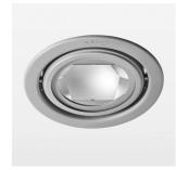
Recessed luminaire with LED, rated life of the LED L80/B10 > 50000 h, colour rendering index CRI > 80, chromaticity tolerance 2 SDCM (initial), reflector with oval light distribution pattern, reflector pure aluminium 99,99% in MIRO-Silver®, swivel angle +25°/-25°, luminaire housing sheet steel, powdercoated, stratosilver, separate driver unit
