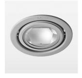
Recessed luminaire with LED, rated life of the LED L80/B10 > 50000 h, colour rendering index CRI > 80, chromaticity tolerance 3 SDCM (initial), reflector with oval light distribution pattern, reflector pure aluminium 99,99% in MIRO-Silver®, swivel angle +25°/-25°, luminaire housing sheet steel, powder-coated, stratosilver, separate driver unit
