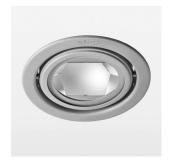
Recessed luminaire with LED, rated life of the LED L80/B10 > 50000 h, colour rendering index CRI > 90, chromaticity tolerance 2 SDCM (initial), reflector with oval light distribution pattern, reflector pure aluminium 99,99% in MIRO-Silver®, swivel angle +25°/-25°, luminaire housing sheet steel, powdercoated, stratosilver, separate driver unit
