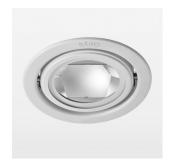
Recessed luminaire with LED, rated life of the LED L80/B10 > 50000 h, colour rendering index CRI > 90, chromaticity tolerance 2 SDCM (initial), reflector with oval light distribution pattern, reflector pure aluminium 99,99% in MIRO-Silver®, swivel angle +25°/-25°, luminaire housing sheet steel, powder-coated, stratowhite, separate driver unit
