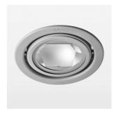
Recessed luminaire with LED, rated life of the LED L80/B10 > 50000 h, colour rendering index CRI > 80, chromaticity tolerance 2 SDCM (initial), reflector with circular light distribution pattern, reflector pure aluminium 99,99% in MIRO-Silver®, swivel angle  $+25^{\circ}/-25^{\circ}$ , luminaire housing sheet steel, powder-coated, stratosilver, separate driver unit
