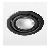
Recessed luminaire with LED, rated life of the LED L80/B10 > 50000 h, colour rendering index CRI > 80, chromaticity tolerance 3 SDCM (initial), reflector with circular light distribution pattern, reflector pure aluminium 99,99% in MIRO-Silver®, swivel angle +25°/-25°, luminaire housing sheet steel, powder-coated, stratoblack, separate driver unit
