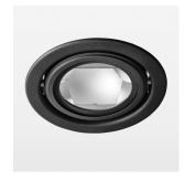
Recessed luminaire with LED, rated life of the LED L80/B10 > 50000 h, chromaticity tolerance 3 SDCM (initial), reflector with circular light distribution pattern, reflector pure aluminium 99,99% in MIRO-Silver®, swivel angle +25°/-25°, luminaire housing sheet steel, powder-coated, stratoblack, separate driver unit
