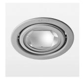
Recessed luminaire with LED, rated life of the LED L80/B10 > 50000 h, colour rendering index CRI > 80, chromaticity tolerance 3 SDCM (initial), reflector with circular light distribution pattern, reflector pure aluminium 99,99% in MIRO-Silver®, swivel angle +25°/-25°, luminaire housing sheet steel, powder-coated, stratosilver, separate driver unit
