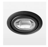
Recessed luminaire with LED, rated life of the LED L80/B10 > 50000 h, chromaticity tolerance 2 SDCM (initial), reflector with circular light distribution pattern, reflector pure aluminium 99,99% in MIRO-Silver®, rotation angle 170°, swivel angle +30°/-30°, luminaire housing sheet steel, powder-coated, stratoblack, separate driver unit
