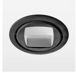
Recessed luminaire with LED, rated life of the LED L80/B10 > 50000 h, chromaticity tolerance 2 SDCM (initial), reflector with asymmetrical light distribution pattern, reflector pure aluminium 99,99% in MIRO-Silver®, rotation angle 170°, swivel angle 15°, luminaire housing sheet steel, powdercoated, stratoblack, separate driver unit
