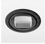
Recessed luminaire with LED, rated life of the LED L80/B10 > 50000 h, chromaticity tolerance 2 SDCM (initial), reflector with asymmetrical light distribution pattern, reflector pure aluminium 99,99% in MIRO-Silver®, rotation angle 170°, swivel angle 15°, luminaire housing sheet steel, powdercoated, stratoblack, separate driver unit
