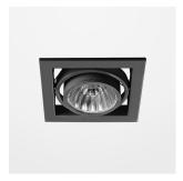
Recessed luminaire with LED, rated life of the LED L80/B10 > 50000 h, colour rendering index CRI > 90, chromaticity tolerance 2 SDCM (initial), reflector with circular light distribution pattern, reflector pure aluminium 99,99% in MIRO-Silver®, cardanic, swivel angle +30°/-30°, luminaire housing sheet steel, powder-coated, stratoblack, separate driver unit
