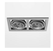
Recessed luminaire with LED, rated life of the LED L80/B10 > 50000 h, colour rendering index CRI > 90, chromaticity tolerance 2 SDCM (initial), reflector with circular light distribution pattern, reflector pure aluminium 99,99% in MIRO-Silver®, cardanic, swivel angle +30°/-30°, luminaire housing sheet steel, powder-coated, stratoblack, separate driver unit
