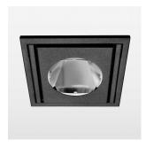
Recessed luminaire with LED, rated life of the LED L80/B10 > 50000 h, chromaticity tolerance 2 SDCM (initial), reflector with circular light distribution pattern, reflector pure aluminium 99,99% in MIRO-Silver®, swivel angle 30°, luminaire housing sheet steel, powder-coated, stratoblack, separate driver unit
