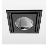
Recessed luminaire with LED, rated life of the LED L80/B10 > 50000 h, chromaticity tolerance 3 SDCM (initial), reflector with circular light distribution pattern, reflector pure aluminium 99,99% in MIRO-Silver®, swivel angle 30°, luminaire housing sheet steel, powder-coated, stratoblack, separate driver unit
