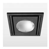
Recessed luminaire with LED, rated life of the LED L80/B10 > 50000 h, chromaticity tolerance 2 SDCM (initial), reflector with oval light distribution pattern, reflector pure aluminium 99,99% in MIRO-Silver®, swivel angle 30°, luminaire housing sheet steel, powder-coated, stratoblack, separate driver unit
