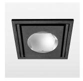
Recessed luminaire with LED, rated life of the LED L80/B10 > 50000 h, chromaticity tolerance 3 SDCM (initial), reflector with oval light distribution pattern, reflector pure aluminium 99,99% in MIRO-Silver®, swivel angle 30°, luminaire housing sheet steel, powder-coated, stratoblack, separate driver unit
