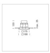
Recessed luminaire with LED, rated life of the LED L80/B10 > 50000 h, chromaticity tolerance 3 SDCM (initial), reflector with circular light distribution pattern, reflector pure aluminium 99,99% in MIRO-Silver®, swivel angle 30°, luminaire housing sheet steel, powder-coated, stratoblack, separate driver unit
