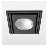
Recessed luminaire with LED, rated life of the LED L80/B10 > 50000 h, colour rendering index CRI > 80, chromaticity tolerance 3 SDCM (initial), reflector with oval light distribution pattern, reflector pure aluminium 99,99% in MIRO-Silver®, swivel angle 30°, luminaire housing sheet steel, powder-coated, stratoblack, separate driver unit
