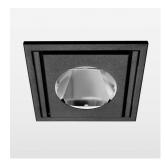
Recessed luminaire with LED, rated life of the LED L80/B10 > 50000 h, colour rendering index CRI > 80, chromaticity tolerance 3 SDCM (initial), reflector with circular light distribution pattern, reflector pure aluminium 99,99% in MIRO-Silver®, swivel angle 30°, luminaire housing sheet steel, powder-coated, stratoblack, separate driver unit
