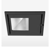
Recessed luminaire with LED, rated life of the LED L80/B10 > 50000 h, colour rendering index CRI > 96, chromaticity tolerance 2 SDCM (initial), reflector with asymmetrical light distribution pattern, reflector pure aluminium 99,99% in MIRO-Silver®, swivel angle 30°, luminaire housing sheet steel, powdercoated, stratoblack, separate driver unit
