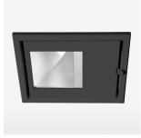
Recessed luminaire with LED, rated life of the LED L80/B10 > 50000 h, colour rendering index CRI > 96, chromaticity tolerance 3 SDCM (initial), reflector with asymmetrical light distribution pattern, reflector pure aluminium 99,99% in MIRO-Silver®, swivel angle 30°, luminaire housing sheet steel, powdercoated, stratoblack, separate driver unit
