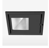
Recessed luminaire with LED, rated life of the LED L80/B10 > 50000 h, colour rendering index CRI > 96, chromaticity tolerance 3 SDCM (initial), reflector with asymmetrical light distribution pattern, reflector pure aluminium 99,99% in MIRO-Silver®, swivel angle 30°, luminaire housing sheet steel, powder-coated, stratoblack, separate driver unit
