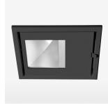
Recessed luminaire with LED, rated life of the LED L80/B10 > 50000 h, colour rendering index CRI > 90, chromaticity tolerance 2 SDCM (initial), reflector with asymmetrical light distribution pattern, reflector pure aluminium 99,99% in MIRO-Silver®, swivel angle 30°, luminaire housing sheet steel, powdercoated, stratoblack, separate driver unit
